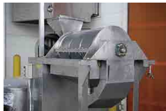
Pulper Finisher for Apple Pure and Tomato Paste (Material : SUS316L) Hole Diameter : 500µm, Plate Thickness : 1.5mm (0.059 inch)
