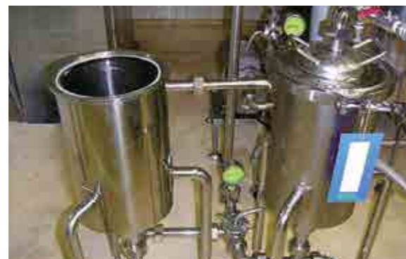
Yogurt Production Line Basket Filter (Material : SUS316L) Hole Diameter : 150µm, Plate Thickness : 0.8mm (0.031 inch)
