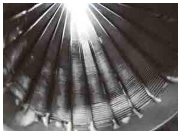
Inner structure of wedge wire filter
