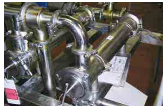
Margarine Production Line Medium-Pressure Line Strainer, Withstand Pressure : 284psi (1.96MPa) Hole Diameter : 500µm, Plate Thickness : 1.5mm (0.059 inch)
