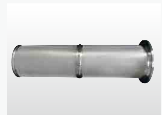
Yeast Paste Production Line Basket Filter (Material : SUS316L) Hole Diameter : 600µm, Plate Thickness : 2.0mm/3.0mm (0.079/0.12 inch)
