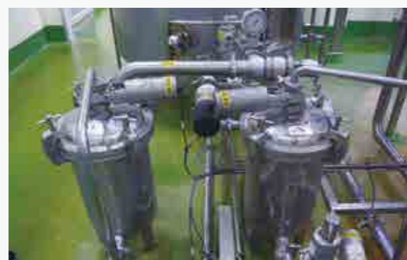
Canned Coffee Production Line Basket Filter (Material : SUS316L) Hole Diameter : 380µm, Plate Thickness : 1.0mm/1.5mm (0.039/0.059 inch)
