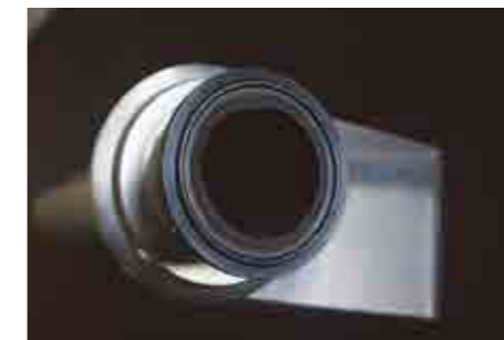
With the rubber tube set in place Rubber tube set into the inside of the filter and water pressure applied
