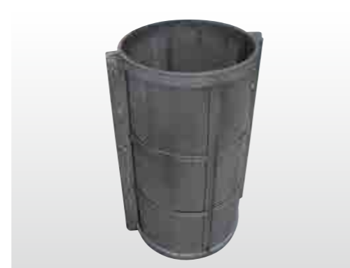
Pulper Finisher for Apple Pure and Tomato Paste (Material : SUS316L) Hole Diameter : 500µm, Plate Thickness : 1.5mm (0.059 inch)
