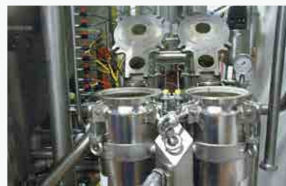
Yeast Paste Production Line Basket Filter (Material : SUS316L) Hole Diameter : 600µm, Plate Thickness : 2.0mm/3.0mm (0.079/0.12 inch)
