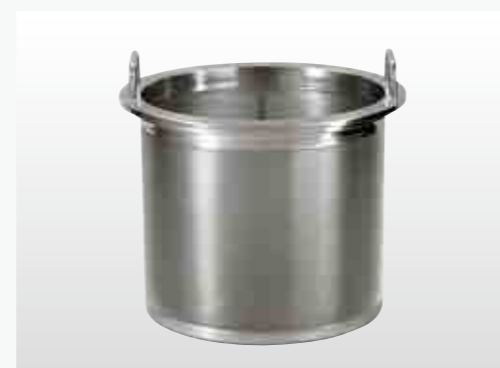
Canned Coffee Production Line Basket Filter (Material : SUS316L) Hole Diameter : 380µm, Plate Thickness : 1.0mm/1.5mm (0.039/0.059 inch)
